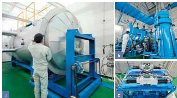
a/ Temperature control chamber b/ Hydraulic pressure cycle test system for 500 L class storage tanks c/ High-temperature creep test equipment
