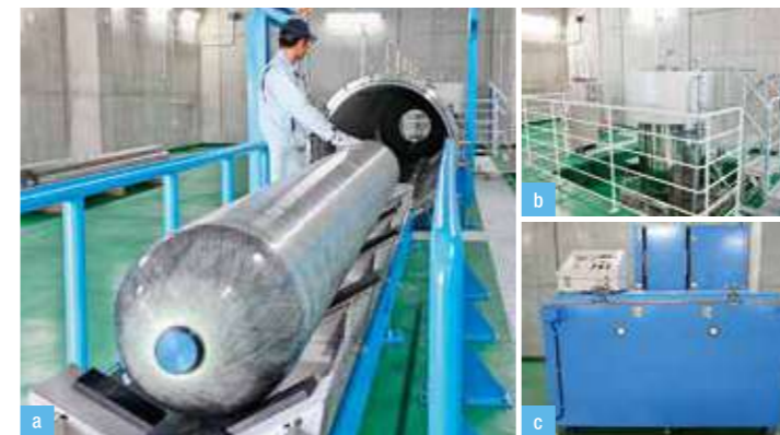
a/ Expansion measurement test system (open) b/ Expansion measurement test system (100 L) c/ Constant temperature over for creep test of a tank
