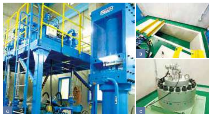
a/ Hydraulic pressure cycle test equipment (300L) b/ Testing pit c/ Pressurization vessel
