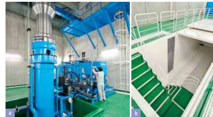
a/ Hydraulic pressure cycle test system for 500 L class storage tanks b/ Testing pit
