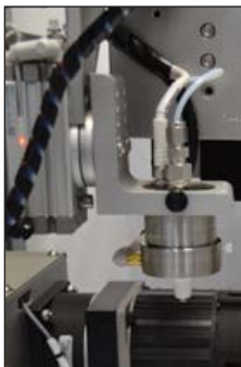
Combined nozzle tilt and rotate option
