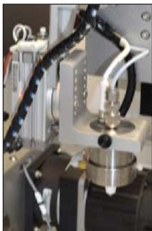
Combined nozzle tilt and rotate option
