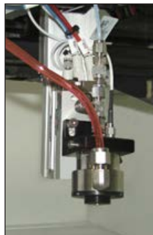
Nozzle two-position pneumatic tilt option
