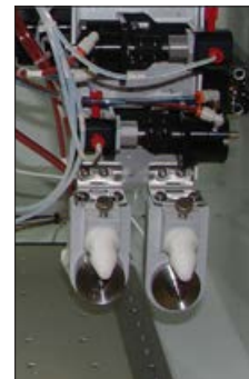
Nozzle two-position rotate option
