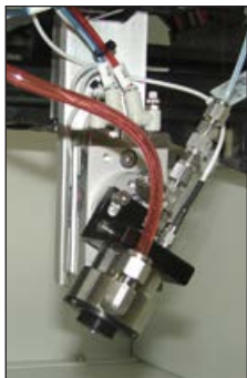
Nozzle two-position pneumatic tilt option
