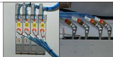
(4) Vacuum Generators - Integrated vacuum pressure gauges allow individual zone pressures to be set.
